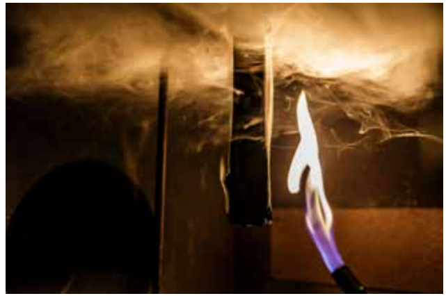
Rubber splice materials should have equivalent resistance properties.
