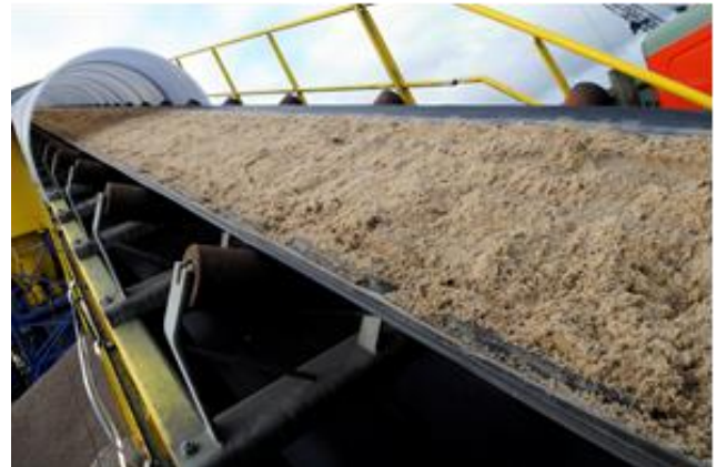
Misaligned drums and idlers cause extra wear
