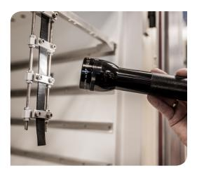
**Right:** Checking for cracks every two hours.
