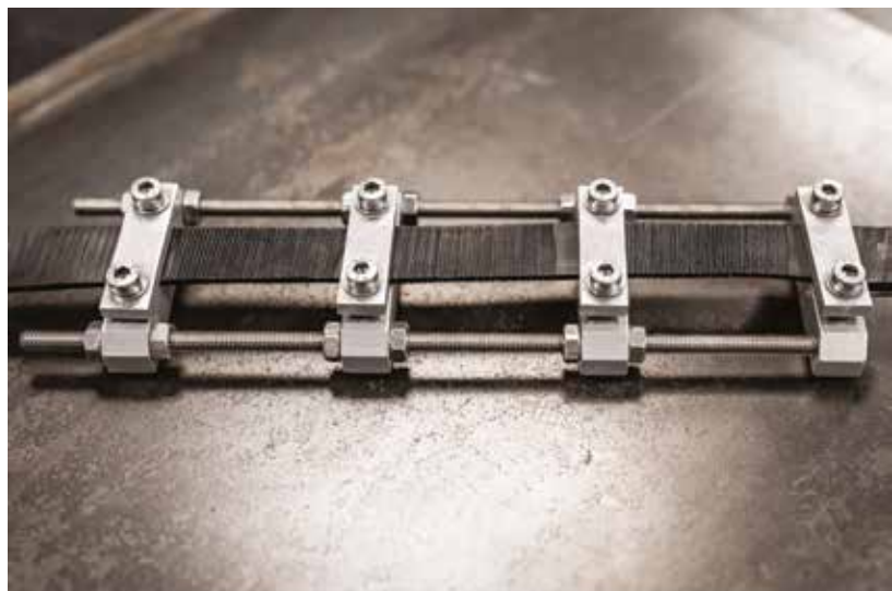
The invisible belt destroyer. The test sample shows serious lateral cracking following exposure to ozone. (EN/ISO 1431 testing)
