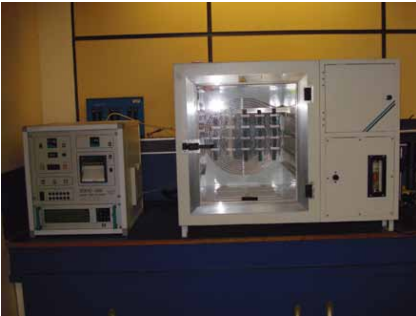
Dunlop's ozone testing cabinet.
