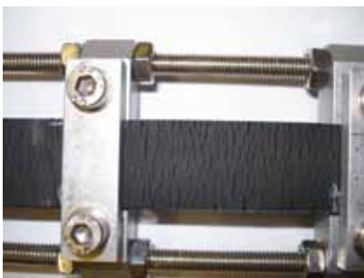
Competitor's belt sample showing surface cracking
