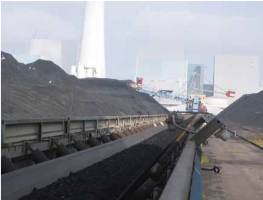
Environment issue? Coal dust can be shaken out from the underside of the belt.
