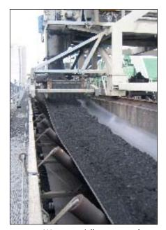
**Fig. 3:** Wear especially occurs at the loading point where the belt is exposed to impact.
