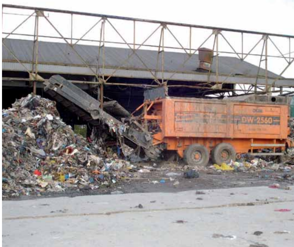
Above: Sharp objects cut and gouge the surface of the belt, which causes the belt to break apart; sometimes literally at the seams. Below: Even general household waste can be a 'belt killer'.
