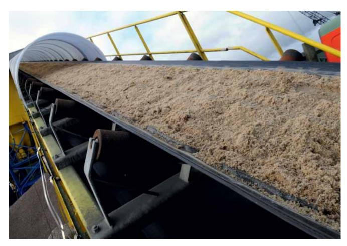
wear caused by abrasion (the most commonly used type), tearing and cutting, heat, fire and oil penetration. These different covers are generally referred to as 'cover grade qualities'.
