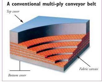
An outer cover of rubber protects the belt carcass. Different types of rubber compound are used for rubber multi-ply belting covers; each designed to withstand damaging effects such as
