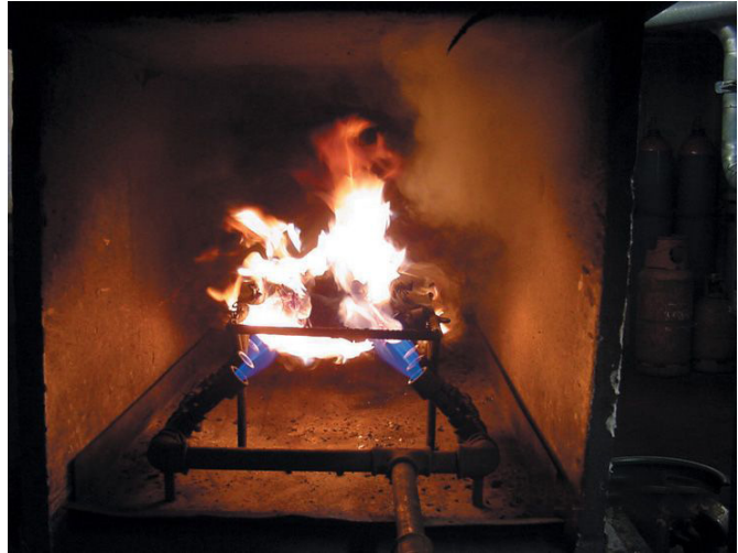
Figure 3. Fire simulation test method EN 12881-1 Method C.
