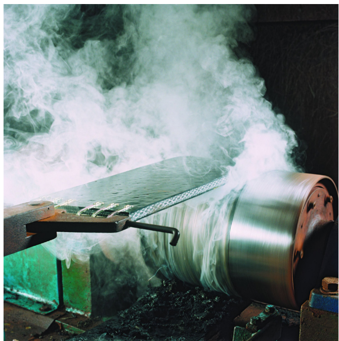
Figure 6. A PVC solid woven belt undergoing drum friction testing.
