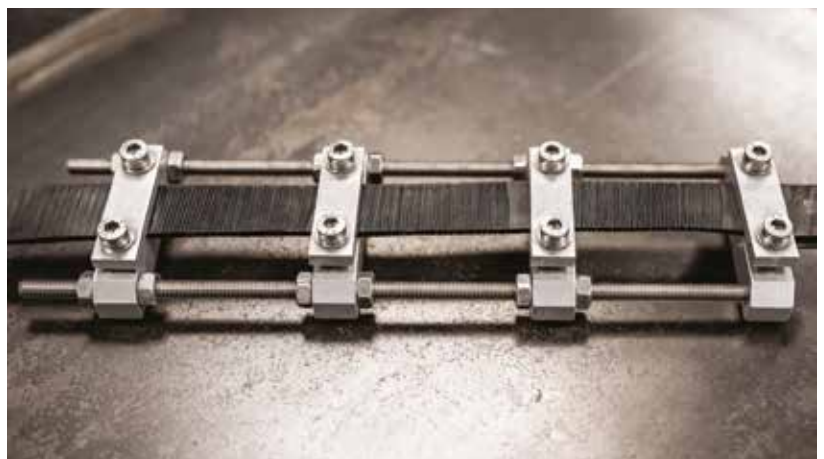
The invisible belt destroyer. The test sample shows serious lateral cracking following exposure to ozone. (EN/ISO 1431 testing)
