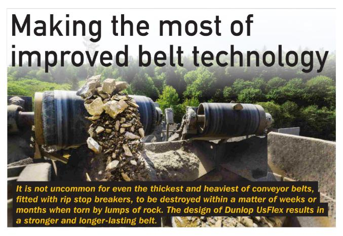
hen faced with the need to repeatedly repair damaged belts and, ultimately, to prematurely replace a barely worn belt, the most obvious answer would seem to be to fit an even heavier, thicker belt, which is very rarely the best solution due to the limitations in pulley diameter, or to fit 'sacrificial' belts but with all the associated issues that frequent belt changes entail
