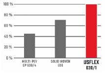
The longitudinal ripping of a conveyor belt is caused when sharp foreign objects penetrate the moving belt and then become trapped. In laboratory tests we pierce a belt with a sharp hook and pull the belt to simulate the ripping action, the force of which is then measured. Such testing consistently shows that the rip resistance of UsFlex is over five times that of conventional multi-ply belts with a similar tensile strength and far superior to Solid Woven and EpP constructions.
