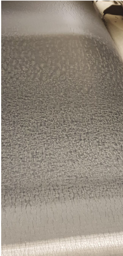
Rubber with poor ozone and UV resistance cracks and degrades prematurely
