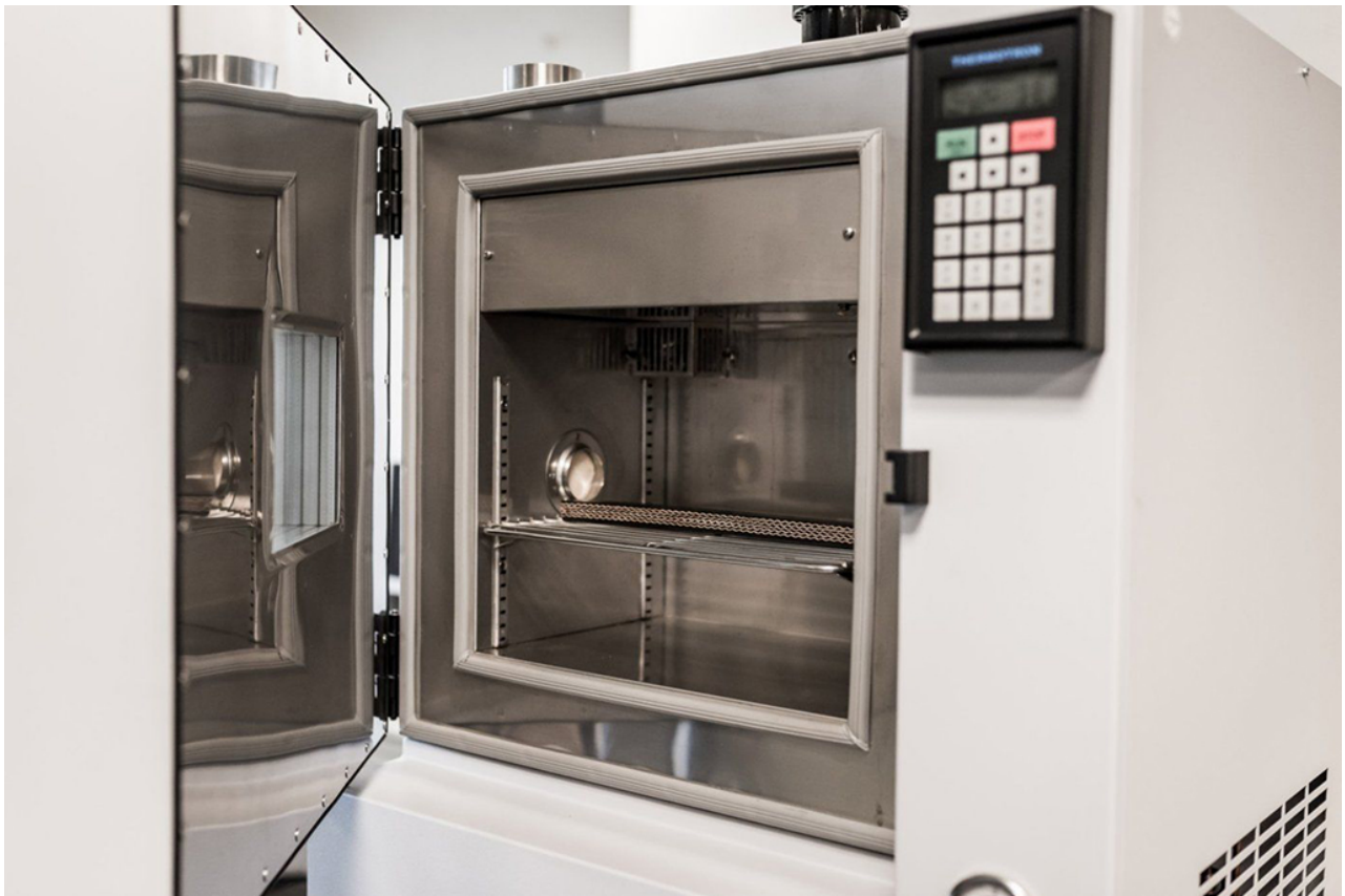
Belt samples are frozen using liquid nitrogen
