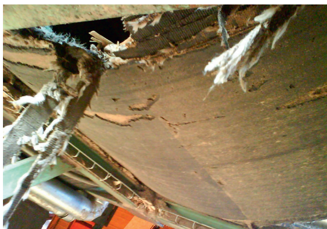
Badly damaged belt (above): Dunlop's abrasion testing (below)
