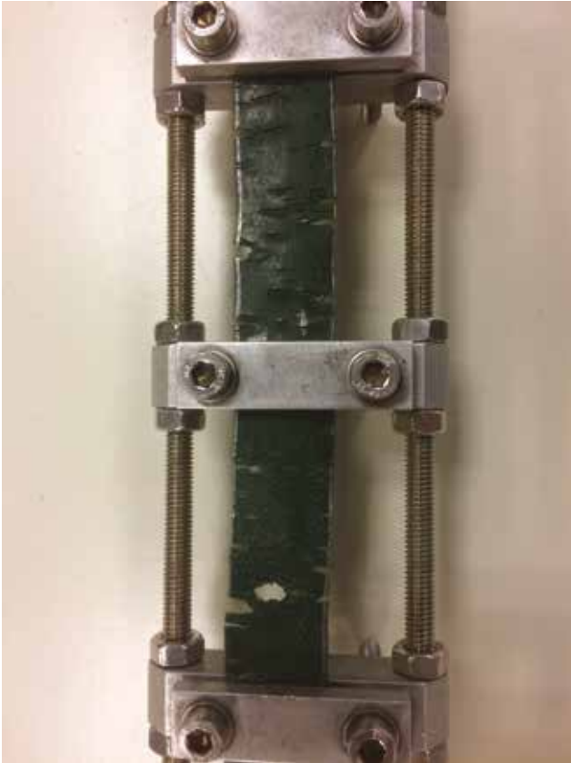
Ozone & UV can rapidly destroy a rubber belt
