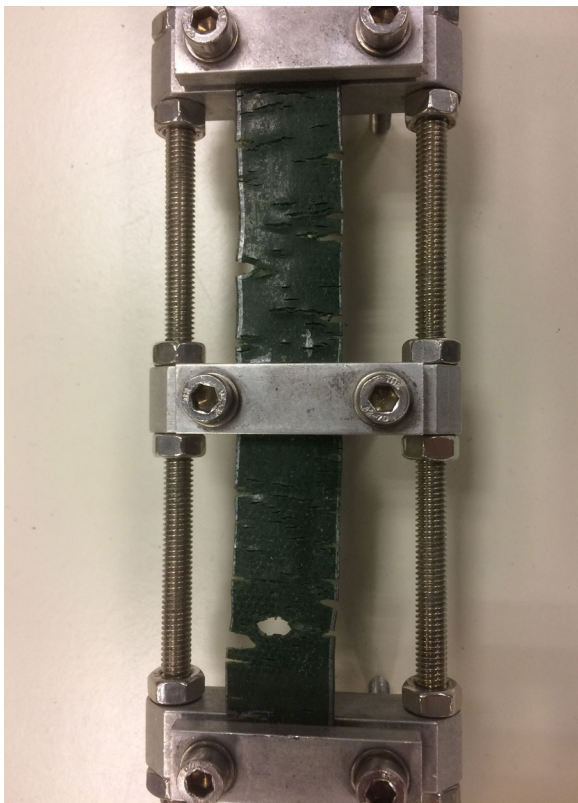
Ozone & UV can rapidly destroy a rubber belt.
