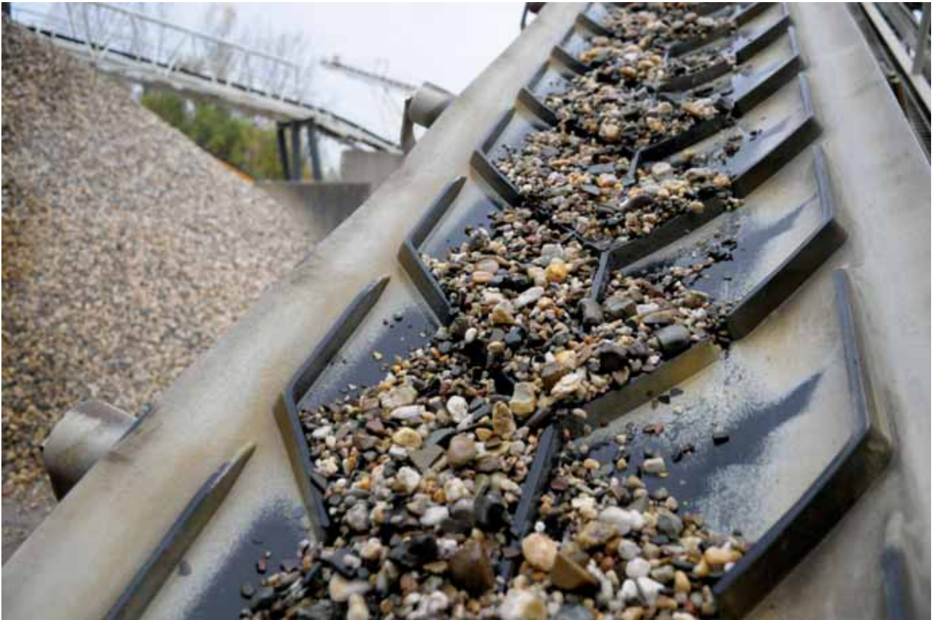
A common problem – profiles that split and eventually detach from the base belt.
