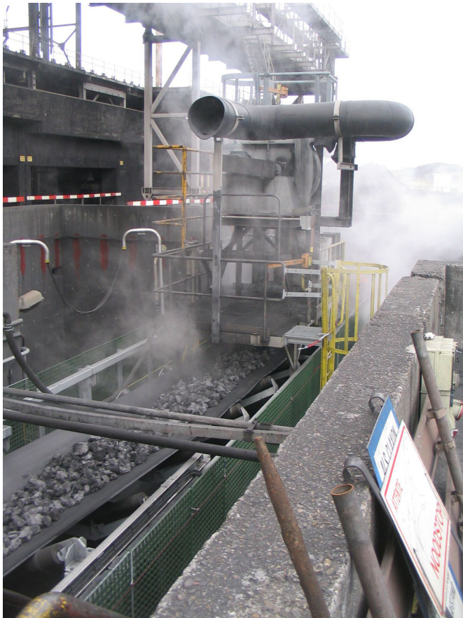
The best of both worlds – Dunlop Betahete exceeds ISO 4195 class T150 requirements and has an average abrasion resistance that is better than DIN X (ISO 14890 'H').
