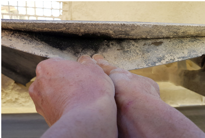
Delamination – the layers of the belt detach themselves.
