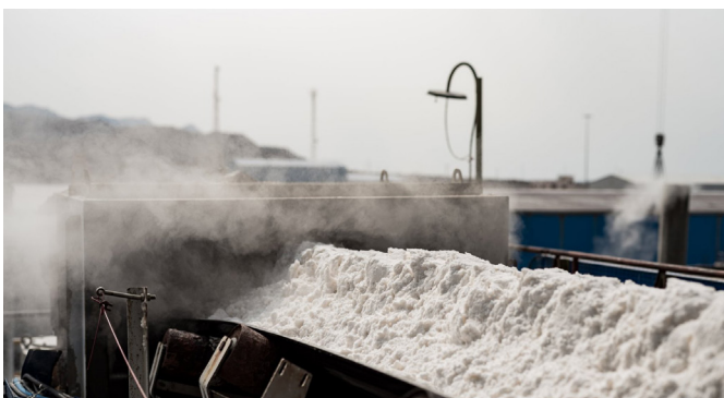
Avoid overloading – uncovered belt surface area allows heat to escape.
