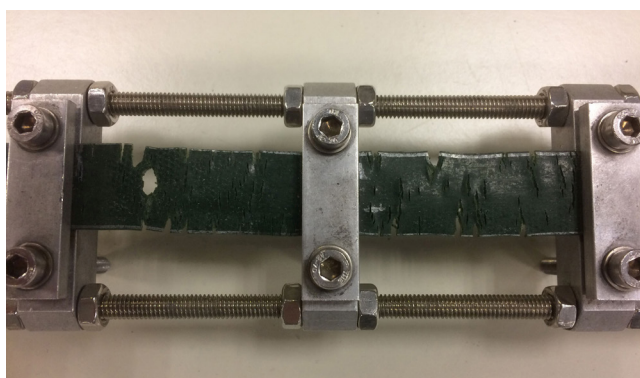
Figure 7. Ozone and UV can rapidly destroy a rubber belt.
