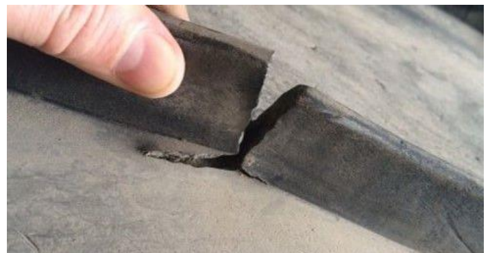
Constant flexing can cause dynamic stress fractures in conventionally produced chevron belts
