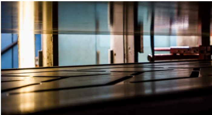
The mould plate used to make a 'Single homogenous structure' chevron belt
