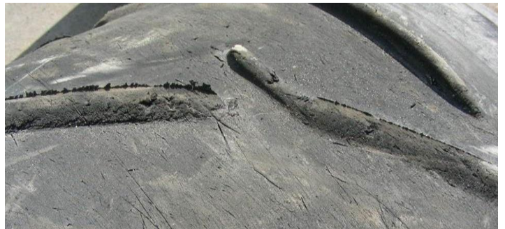
Chevrons as high as 25mm or 32mm can wear almost completely flat in a very short time
