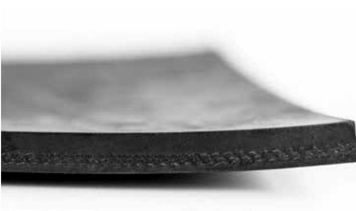
Not what they seem – The use of totally polyester (EE) plies rather than a combination of polyester and nylon.
