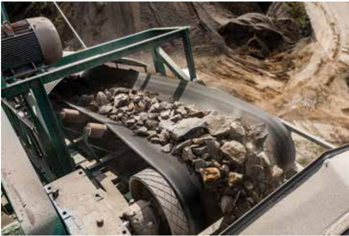
Not what they seem – The use of totally polyester (EE) plies rather than a combination of polyester and nylon.
