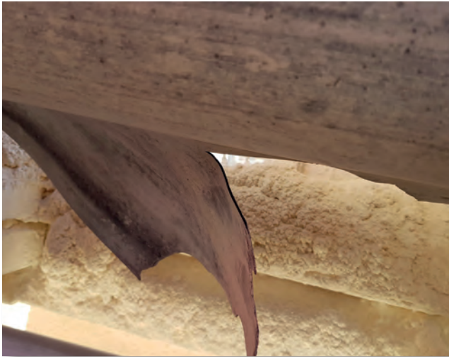
Figure 3: An increase as little as 10 °C in core temperature can cause a belt to fall apart
