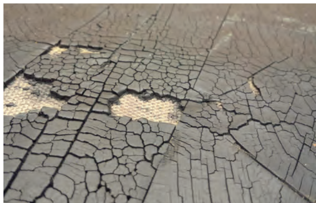
Figure 1: A heat stressed conveyor belt surface
