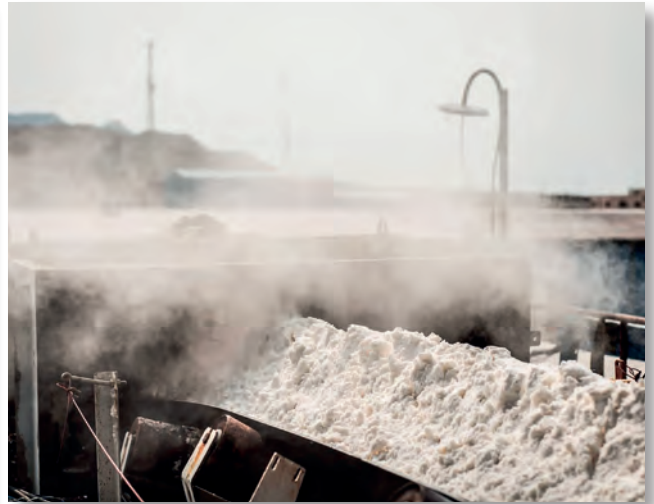
Figure 4: Avoid overloading – uncovered belt surface area allows heat in the belt to escape
