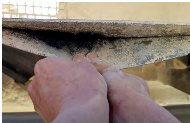
Figure 2: Delamination – the layers of the belt detach themselves
