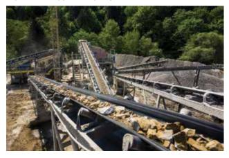
The use of EE fabrics instead of EP reduces troughability, impact resistance and rip resistance.
