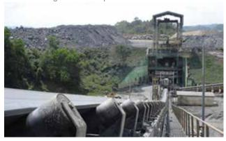
The belt carcass plays a vital role in minimising the effects of impact and trapped sharp objects.
