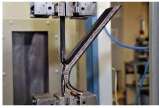
Measuring adhesion literally involves pulling the layers apart and measuring the force required.
