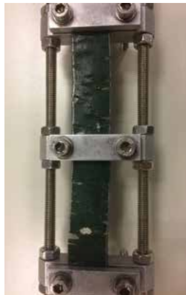
Ozone & ultra violet light causes rubber to literally disintegrate.
