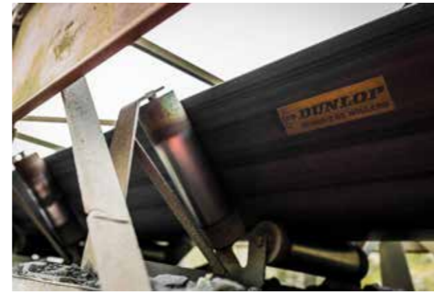
Ripping, tearing and impact – the best solution is to fit a conveyor belt specifically engineered for the purpose.
