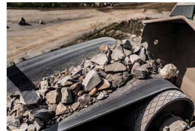
Different causes of wear and abrasion require different kinds of abrasion resistant rubber.
