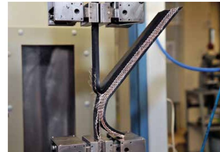
It is a good idea to have a piece of spare belt laboratory tested to measure its true properties.
