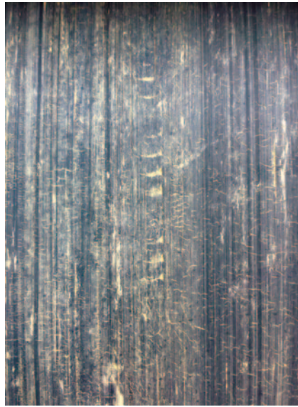
Shorter lifespan – belting imported from Asia is very rarely ozone and UV resistant.
