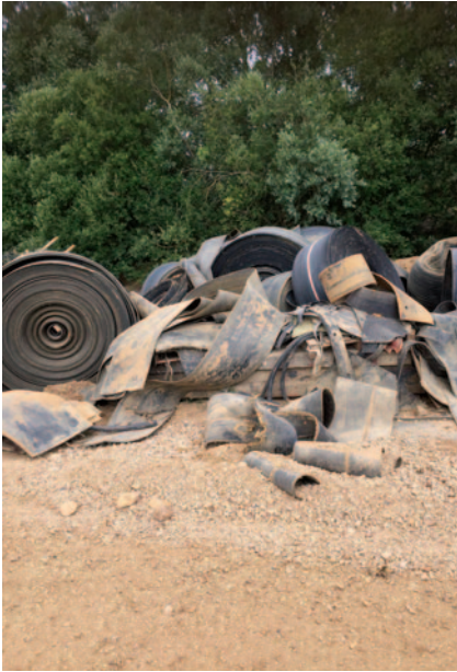
Not the real thing - ruined and worn out multi-ply belting imported from China.
