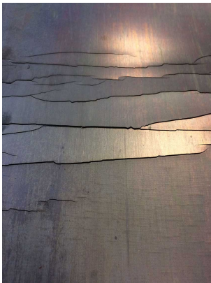
High temperatures create 'accelerated ageing' effects such as the hardening and cracking
