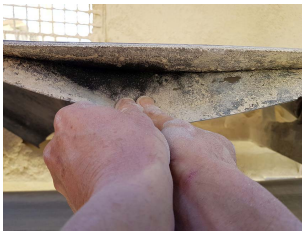
Delamination is a common cause of premature belt replacement
