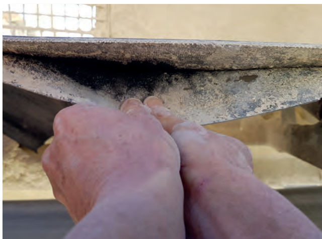
Figure 1: Delamination – the layers of the belt detach themselves
