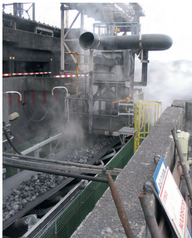
Figure 6: Heat-resistant belts can be capable of lasting two or three times or more longer
