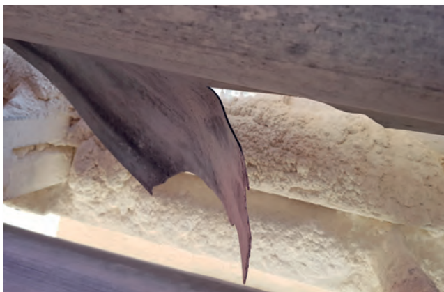
Figure 3: An increase as little as 10 °C in core temperature can cause a belt to fall apart
