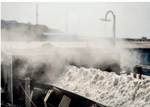
Figure 5: Overloading should be avoided – uncovered belt surface area allows heat to escape
