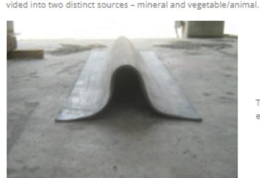
The oil present in biomass can seriously distort even the thickest of conveyor belts
