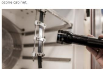
Samples are examined for evidence of cracking at two-hourly intervals
