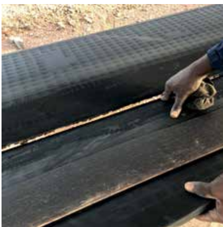
Longitudinal rips are every conveyor operator's nightmare
