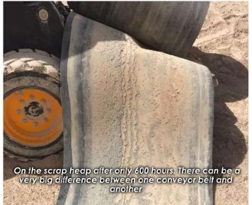
need for frequent repairs and premature replacement. Indeed, all the evidence points to top quality European-made belts being able to provide up to four or five times longer operational life compared to their Asian counterparts. Their cost over their working life is therefore appreciably less.
