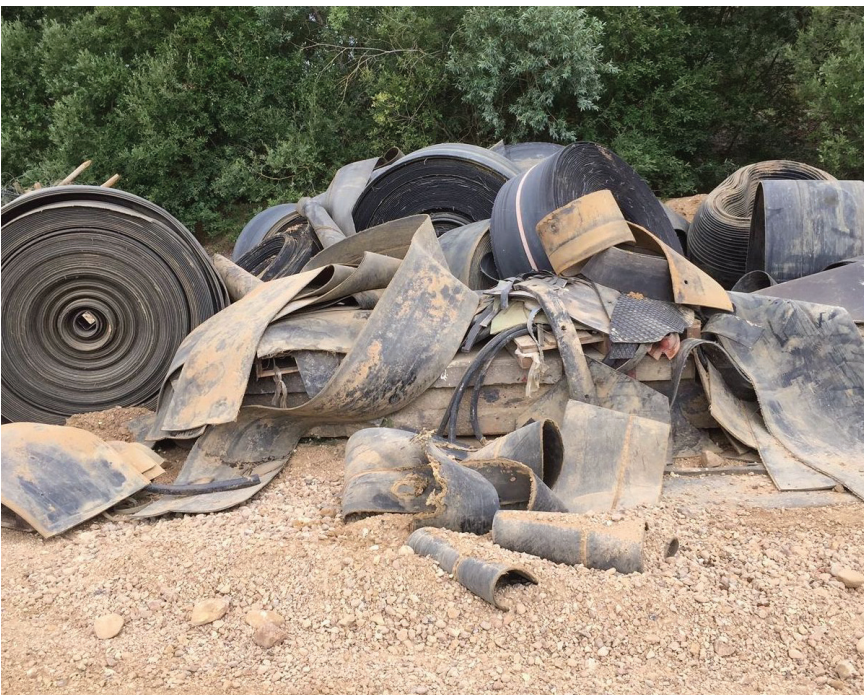
Out with the old – ruined and worn out imported multi-ply belting from the pre-Dunlop days
