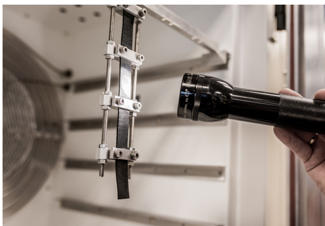
Figure 6. Samples are checked for cracking at two-hourly intervals.
