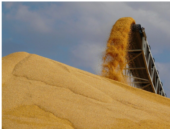
Class 2A is usually perfectly adequate for moderately abrasive materials such as grain.
