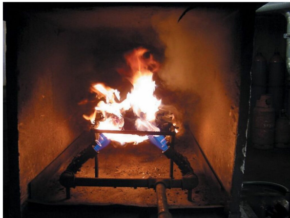
Class 4A entails EN12881-1 method A, C or D in addition to EN/ISO 340 testing
