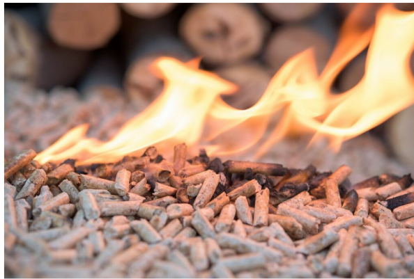
Biomass dust can be prone to self-ignition
