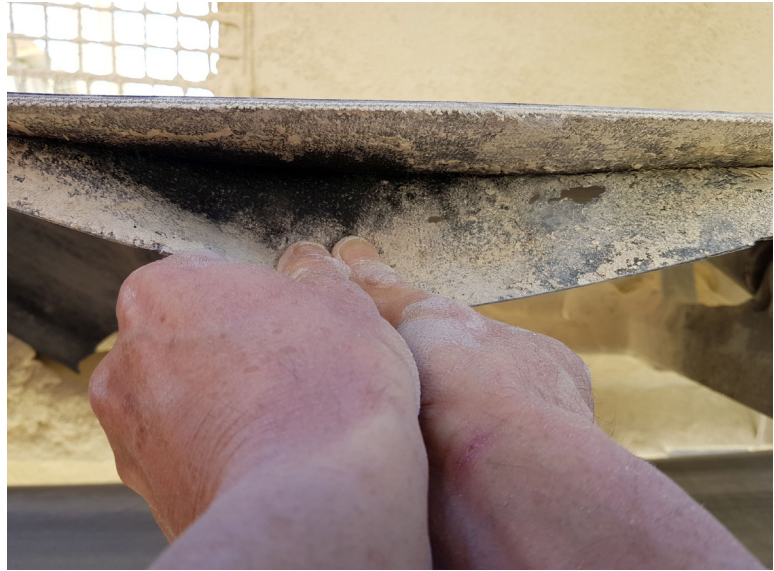
Delamination – the layers of the belt detach themselves.
