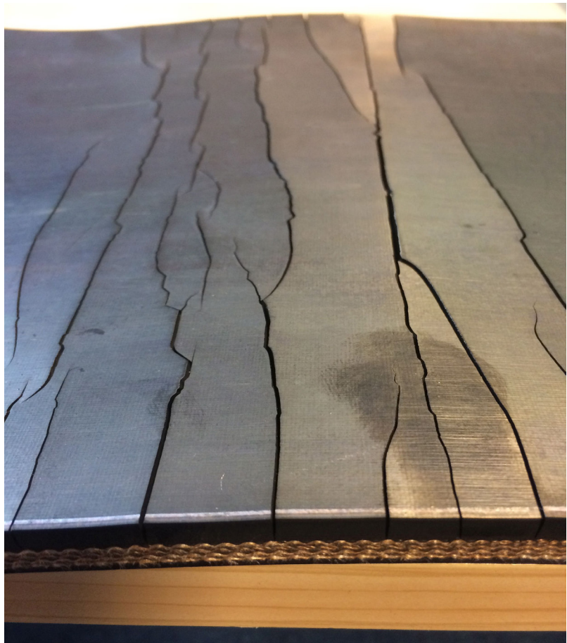
Some crack earlier than others – not all heat-resistant belts perform the same.
