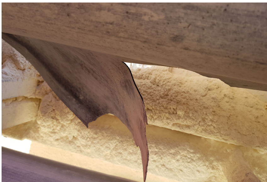
An increase of as little as 10°C in core temperature can cause a belt to fall apart.
