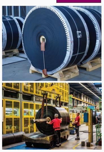
**Lifting:** the recommended method for lifting rolls is to insert a steel core of suitable size with a square cross-section through the reel centre hole. Slings, steel cables or chains suspended from a crane/hoist with beam should be used for fastening. The distance between the fastening points of the steel core sling should be longer than the width of the belt in order to avoid damage to the belt edges.
