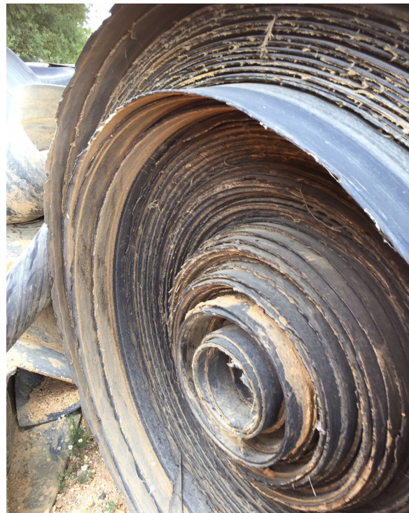
Rubbing against the conveyor structure strains the motor and damages the belt.
