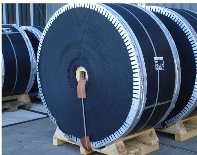
Figure 2. Conveyor belt rubber is almost entirely synthetic.
