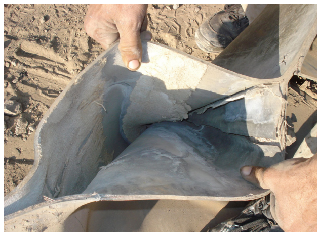
Figure 5. Conveyor belting falling apart – sacrificed on the price altar.
