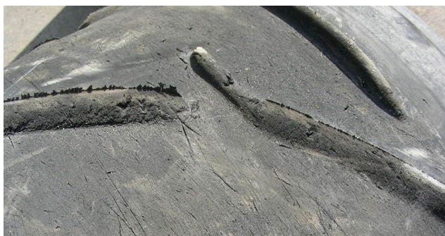
Figure 3. Rapid wear of conveyor rubber.
