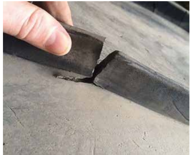
Constant flexing can cause dynamic stress fractures in conventionally produced chevron belts
