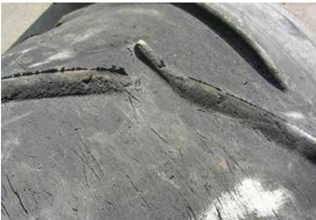
Chevrons as high as 25mm or 32mm can wear almost completely flat in a remarkably short time.
