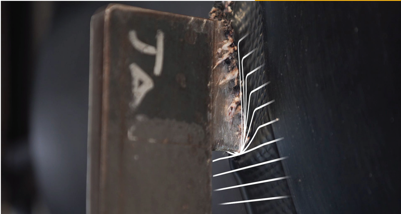
Weft strands bundle together to stop the belt or expel the penetrating object
