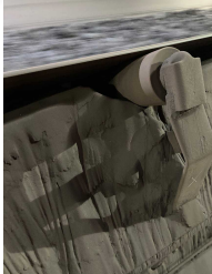
An unclean environment is a common cause of misalignment
