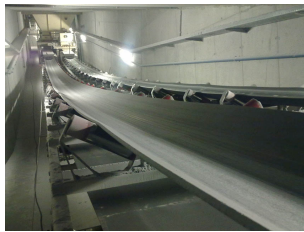
Training a belt when it is empty should mean it will also run true when loaded
