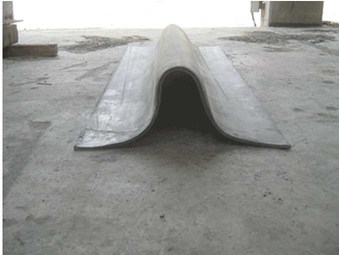
Photo courtesy of Dunop Oil can seriously distort flat rubber belts.
