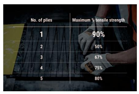
One of the best ways to increase splice reliability is to employ the finger splice method, ideally by changing to the new generation of super-strength single and dual-ply belts pioneered by Fenner Dunlop.
