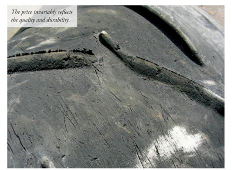
strands of the fabric may be sufficient to achieve the required tensile strength, rip and tear resistance are reduced, and elongation (stretch) is lowered. This in turn can cause problems with transition distances and a general inability to accommodate the contours of the conveyor and its drums and pulleys, ultimately lead to premature failure.
