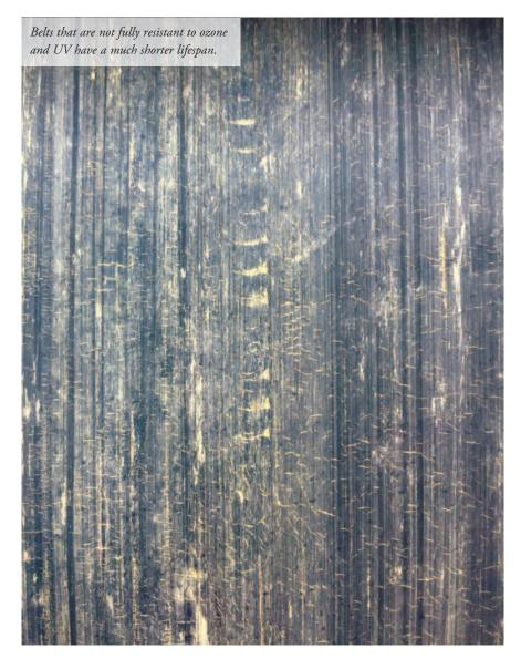
several consequences including surface cracking and a marked decrease in the tensile strength, all of which accelerates the wear and general degradation of the rubber.
