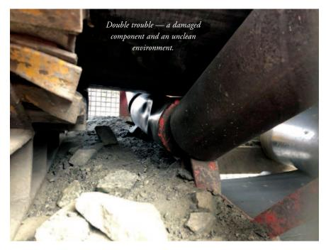
Low-quality rubber and poor adhesion between the inner plies and outer covers are both faults commonly found in the lowgrade belts and make the job difficult even for the most skilled splicer. The cost of splice joint repairs and the associated lost output should always be included when calculating the whole life cost of a conveyor belt.
