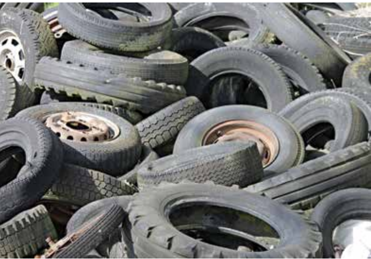
Lower-grade carbon black can be produced cheaply by burning scrap car tyres.
