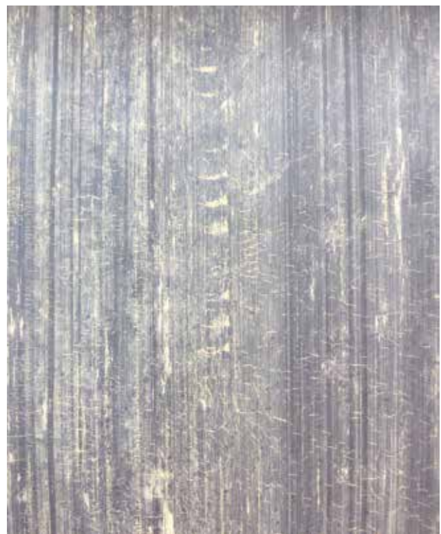
Shorter lifespan – belting imported from Asia is very rarely ozone and UV resistant.
