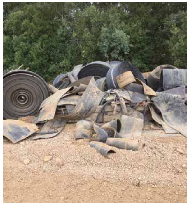
Not the real thing - ruined and worn out multi-ply belting imported from China.
