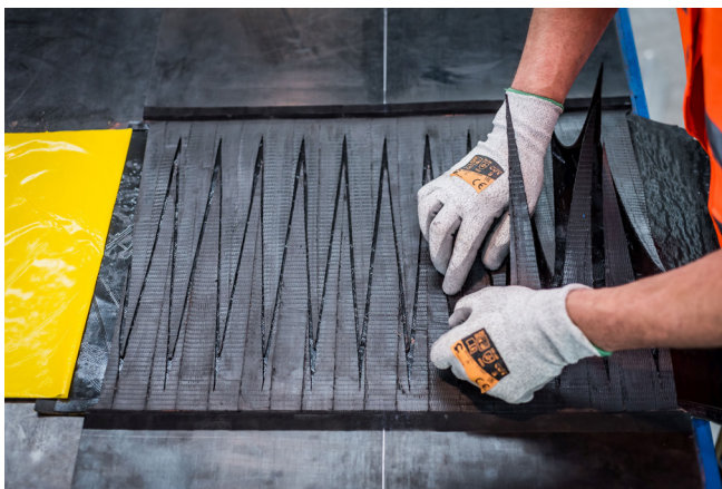
Figure 5. A finger splice may take longer but is stronger and more reliable.
