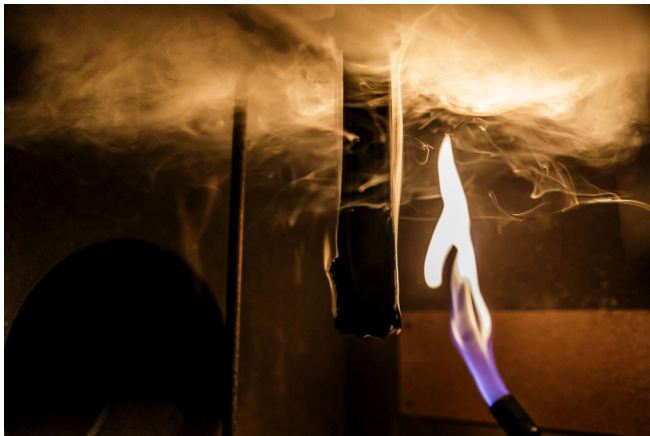
Figure 2. Rubber splice materials should have equivalent resistance to fire, oil, or heat.
