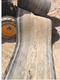
The wear resistance of rubber is a combination of overall strength, resistance to abrasion and resistance to cut and tear propagation.
