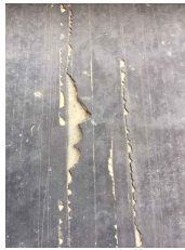
Ozone & ultra violet light causes rubber to crack and break up
