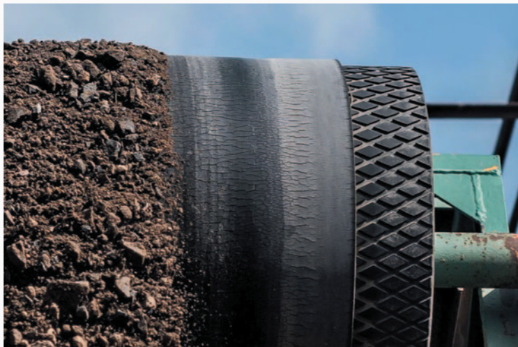
The beginning of the end – cracks can occur within a few months, sometimes only weeks.
