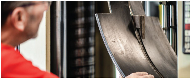
Figure 2. Dunlop's 'Jack the Ripper' rip test in action.
