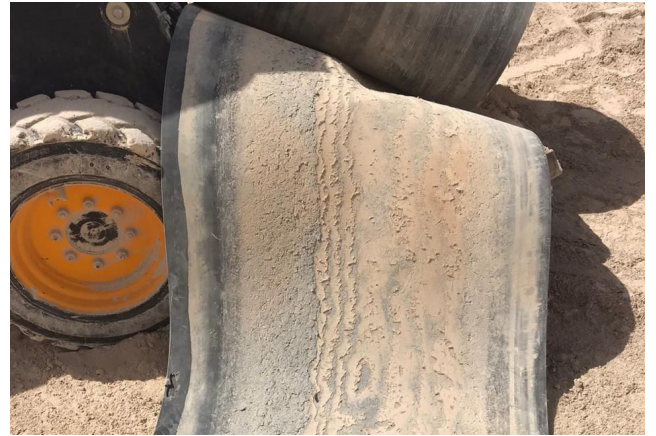
Figure 7. The wear resistance of rubber is a combination of overall strength, resistance to abrasion, and resistance to cut and tear propagation.
