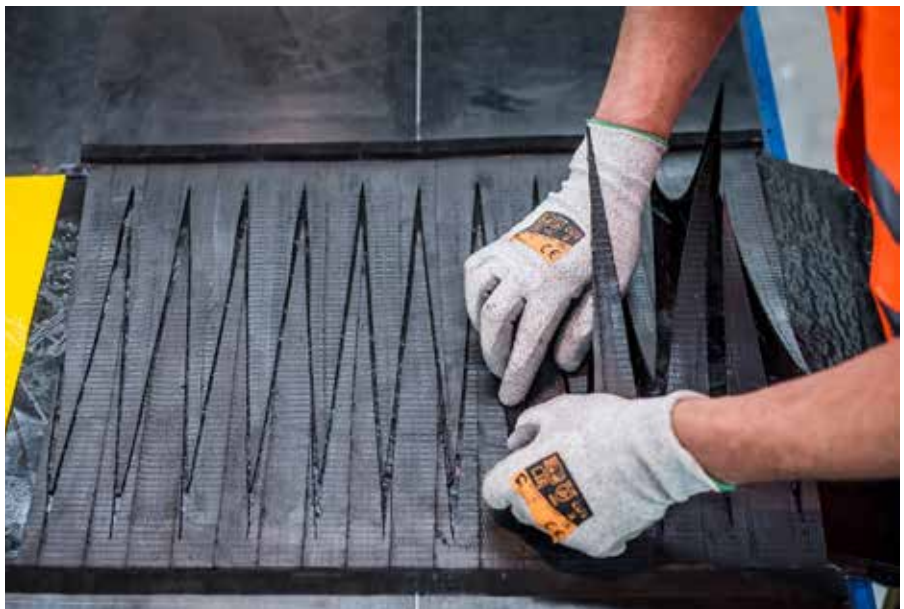
Finger splice joints are stronger and more durable
