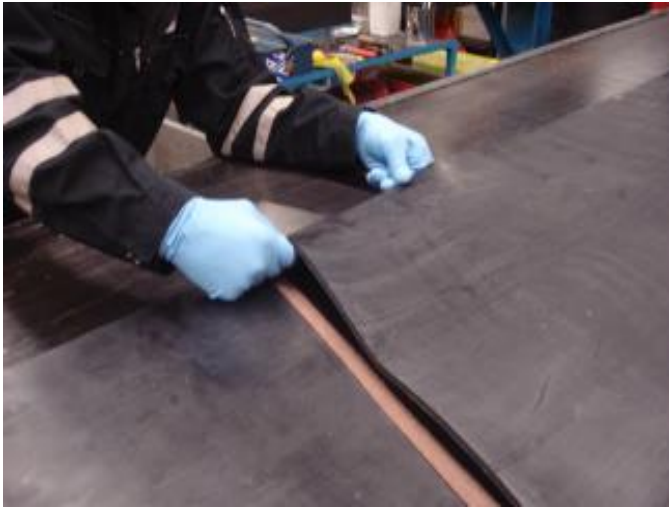
Photo 10. Aligning and matching the belt-ends
