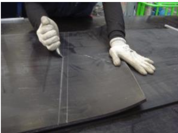
Photo 3. Cutting at an angle of 45°
