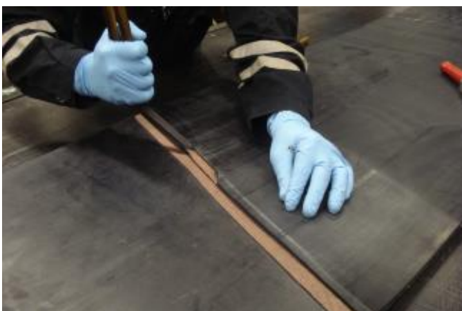
Photo 12. Remove the filler strip
